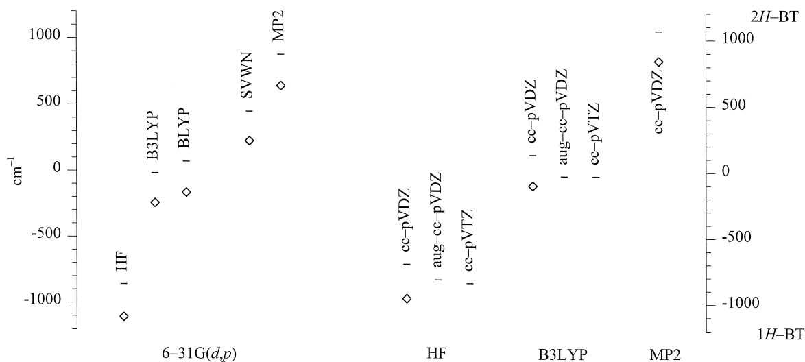
Fig. 2. Relative ab initio stabilization energies of 1H - and 2H -BT for different methods (HF, B3LYP, BLYP, SVWN, MP2) and different basis sets. Up to the MP2 level the stabilization of 2H -BT relative to 1H -BT increases, while with increasing basis set the 1H -tautomer is favoured. The pure electronic stabilization energy \Delta D_e is designated with - , the ZPE corrected value \Delta D_0 with \diamond .
